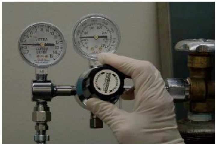
Adjusting the Flow-control knob for either the “mouse” or “rat” setting on the Flow gauge
